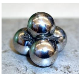
Figure 4. Appearance of weld balls
